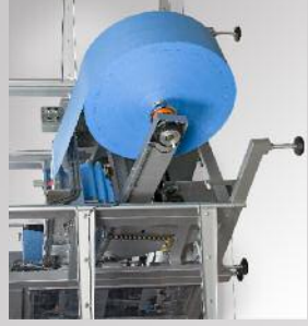
Unwinding of large rolls of up to ø 1,2 m
