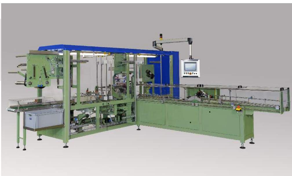
WR 500. Film width 300 mm and film draw-off at 500 mm
