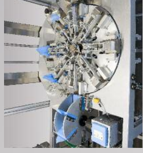
Multi-folding station with a rotary plate
